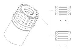
Φ11mm waterproof rubber ring (assembled) suitable for cable OD 9-11mm
