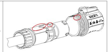
(5) After the assembly of the strain relief, inner core component and housing, tighten the bushing in a clockwise direction with a torque of 2.0 Nm.
